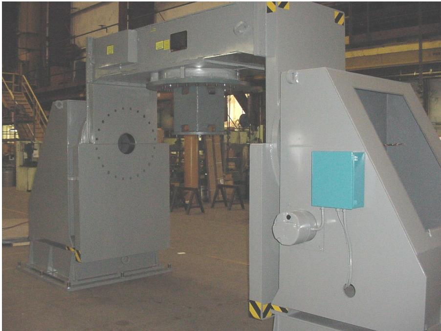
The DCG series Positioner provides 2-axis motion, continuous rotation, and  $\pm 180^\circ$  tilt from the horizontal table position. This configuration of Positioner can also be made in a Geared Elevation version with a third powered axis for elevation. The worktable's surface can be specified at varying distances below the tilt axis, as well as specifying swing radius clearances from the table's rotation axis to the nearest obstruction.
